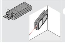
The orientation of the endpiece is automatically detected and the zero point is accordingly adjusted.
